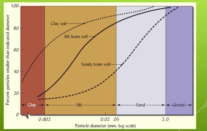
Particle-size distribution in three soils varying widely in their textures. Note that there is a gradual transition in the particle-size distribution in each of these soils.
