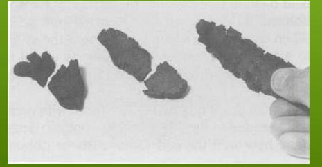
Determination of texture by the field method. Loam soil on left forms a good cast when moist. Clay loam in center forms a ribbon that breaks somewhat easily. Clay on the right forms a long fexible ribbon.
