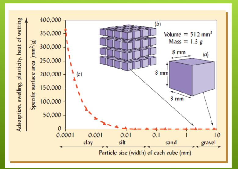
The curve (c) explains why nearly all of the adsorbing power, swelling, plasticity, heat of wetting, and other surface area-related properties are associated with the clay fraction in mineral soils.
