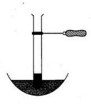
(2) Plunge ignition tube in 10-15 ml distilled water.
